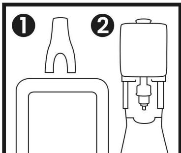
**2** Remove the bottle inside before refilling. DO NOT refill the bottle while it is inside the dispenser.
