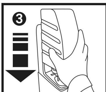
**3** Position the cartridge tip above dispenser opening then lower the cartridge so that it rests safely on the dispensers base.
