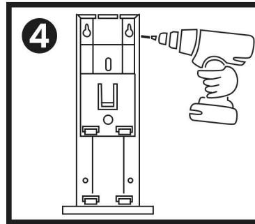
3 Use the separated back plate as a guide to mark the screw location for proper alignment of the screws prior to drilling.
