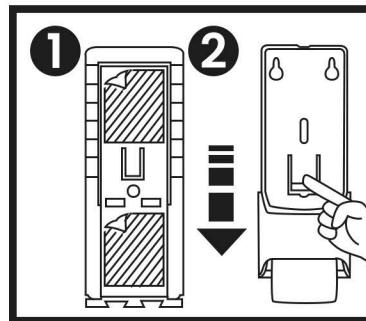
1 Peel away the adhesive tap to expose the screw holes used in mounting the dispenser.
