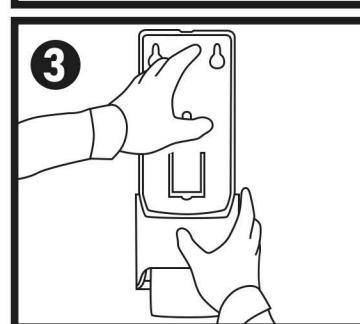
**3** Firmly press the dispenser against the flat surface in the same location that was cleaned with the alcohol wipe.
