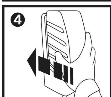
**4** Simply push the cartridge forwards until it touches the back of the dispenser and 'clicks' into place.
