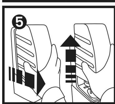
**5** To swap out the cartridge and refill the dispenser, follow steps 1 through 4 as shown up above but in reverse. Pull the cartridge instead of push, and lift instead of lower.
