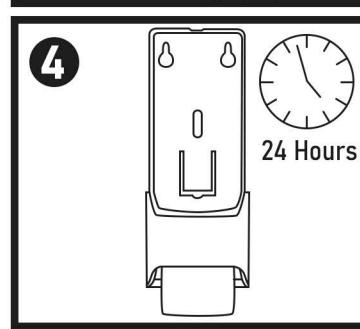
**4** DO NOT place cartridges in the dispenser until 24 hours have passed. This will allow the adhesive tape to solidify before weight is applied.
