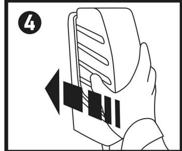
5 To swap out the cartridge and refill the dispenser, follow steps 1 through 4 as shown up above but in reverse. Pull the cartridge instead of push, and lift instead of lower.
