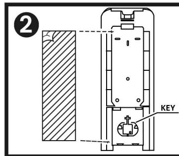
**2** Located on the back of the dispenser, are two square adhesive's with thin covers.
