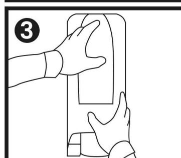
**3** Firmly press the dispenser against the flat surface in the same location that was cleaned with the alcohol wipe.
