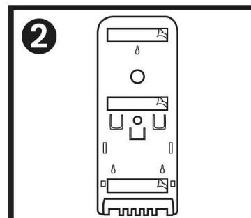
**2** Peel the thin plastic cover protecting the tape on the back of the dispenser.
