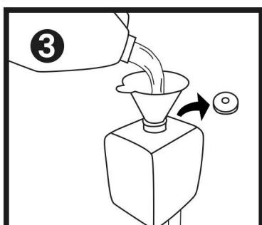
**3** Remove the cap from on top of the bottle. We recommend using a funnel to refill the bottle to help prevent accidental spills.
