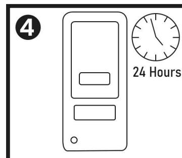
**4** DO NOT fill the dispenser with product until after 24 hours. This will allow the adhesion to solidify before weight is applied.
