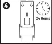
DO NOT fill the dispenser with cartridges until after 24 hours. This will allow the adhesion to solidify before weight is applied.
