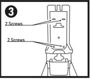
3 The 4 screws provided will go in the marked holes shown in the diagram.
